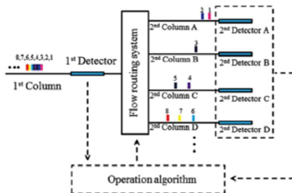
**Diagram of the Fan group's smart 2-D micro-gas chromatography system.** 2-D signifies two levels of separation and detection, and "smart" references an automation algorithm that can route partially separated gas clouds to the appropriate (vacant or specialized) second-level column. Dashed lines represent signal pathways. Source: Lab Chip, 2013, 13, 818 <[tinyurl.com/2DmicroGC](http://tinyurl.com/2DmicroGC)>. Reproduced by permission of The Royal Society of Chemistry.
